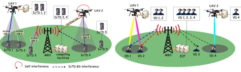
Fig. 7. A novel UAV-assisted mobile edge computing architecture.
