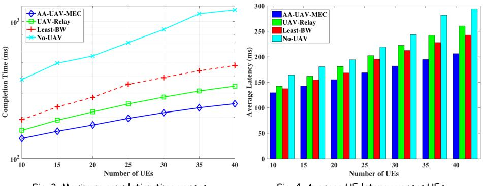
Fig. 3. Maximum completion time versus UEs with three UAVs.
