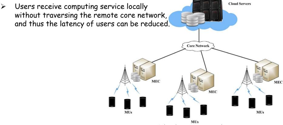
Fig. 1. A mobile edge computing architecture.
